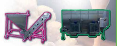
A single Kettle /Coater line that will typically produce 350lbs/hr (160Kg//hr) of Caramel Corn. A twin Kettle/Coater line will produce double that.
